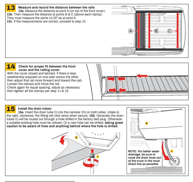
For proper cover operation, ensure rails are positioned correctly (must be parallel). See steps 11 & 12. These surfaces must be level.
