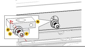
Before tightening the hardware, make sure the top of the RamBox rail is level with the top of the plastic bed rail cap. Do this on the driver and passenger side.
