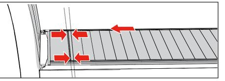
Remove the protective film and install the drain tubes:
