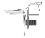
If the rails measured too close together, turn the screws counter clockwise. If the rails measured too far apart,
