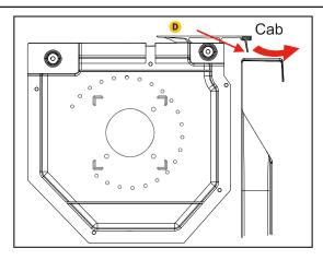
**NOTE:** With the cover in place, the front seal lays flat on the bulkhead, but must not extend past the bed rail cap. Trim the seal as needed to ensure that it lays flat.
