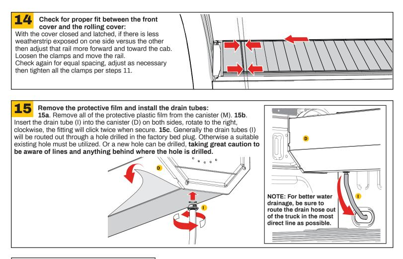
For proper cover operation, ensure rails are positioned correctly (must be parallel). See steps 12 & 13.
