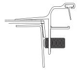
If the rails measured too close together, turn the screws counter clockwise. If the rails measured too far apart,
