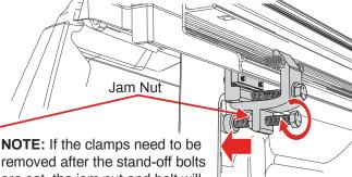
are set, the jam nut and bolt will have to be loosened.
