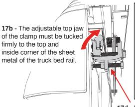
17c - If the jaw does not contact firmly into the corner of the bed flange, remove the clamp and loosen the screws to adjust the
