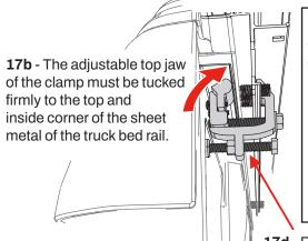
**17c** - If the jaw does not contact firmly into the corner of the bed flange, remove the clamp and loosen the screws to adjust the jaw.
