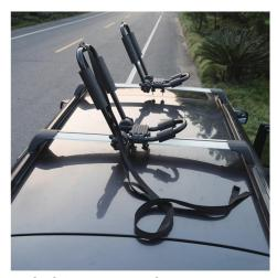
Feed half of the length of the strap into the loop.
