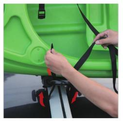
Thread the non-cam end of the strap from underneath the cross bar and pull it out through the shorter arm of the rack.
