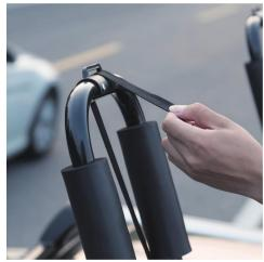
Put the non-cam end of the lashing strap through the plastic loop on the longer arm
