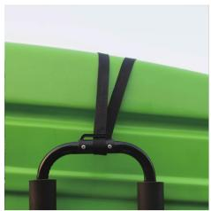
Load the kayak or canoe onto the rack, put the two-fold straps over the kayak.
