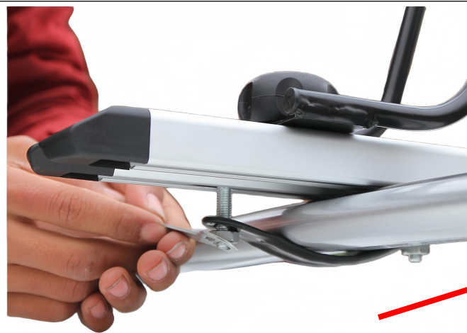
4. Slide 4 T-bolt M8X45mm into the channels under the aluminum bar, and use 2* metal bracket to tight the rear part on the rear crossbar.
