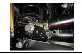
Once the desired length is reached you must tighten and set the jam nut on the adjustable end of track bar.
