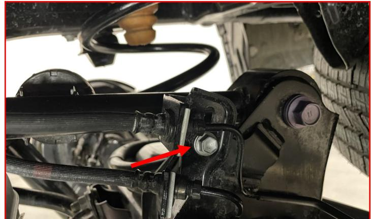
Install the end link onto the frame using **factory hardware**.
