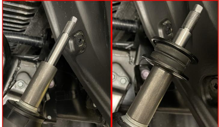
Install the **upper factory shock bushing** and **nut**.
