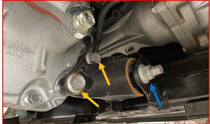
Above the **passenger side bracket**, the differential sensor wire needs to be relocated.
