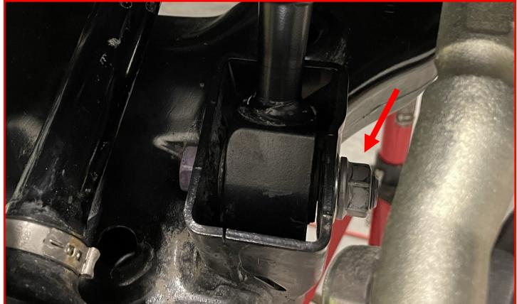
Raise the lower control arm enough to install the upper strut to the perch using the supplied **M10-1.25 serrated flange nuts**.
