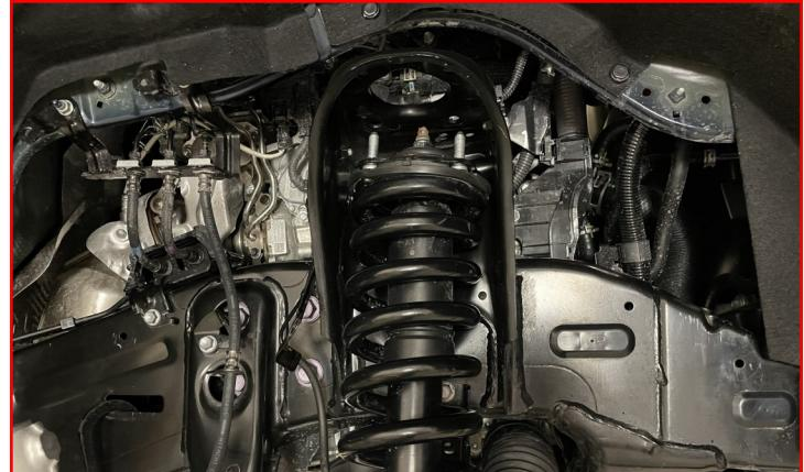
Remove the **lower strut bolt** and let the strut rest in the lower control arm.
