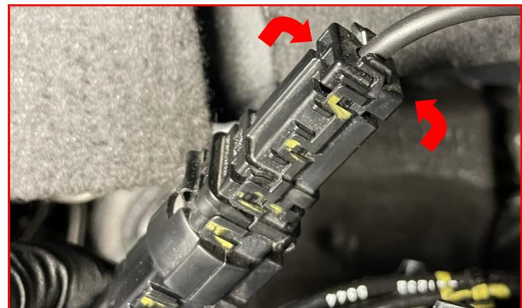
Slide the bracket into the plug housing until it clicks.
