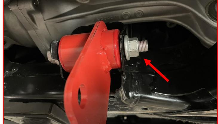
Attach the diff drop bracket to the differential using factory hardware, supplied M16 flat washers, and M16-1.5 C-lock nuts. Note the orientation of the hardware.
