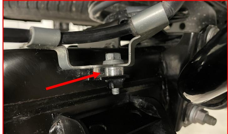
Install the **rear brake line spacer** between the brake line and the chassis using the **factory bolt** (one on each side) holding the brake line to the axle.
