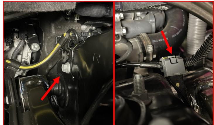
Using **factory hardware** (installed front to back), install the ReadyLift **upper control arm**.
