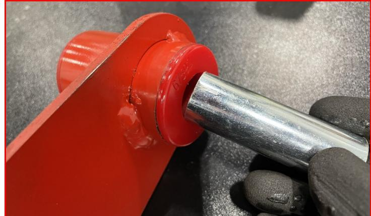
Using **factory hardware**, attach the ReadyLIFT driver diff drop bracket to the chassis.
