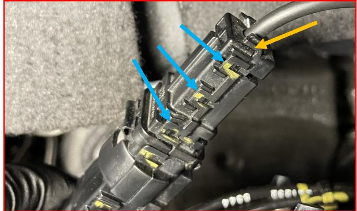
With the plug open, release the **latch** holding the plug pigtail. Remove the plug pigtail.
