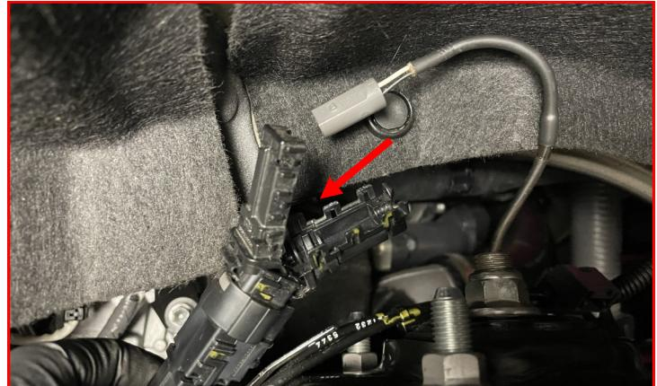
Close the latch on the plug until all six (6) latches click into place.
