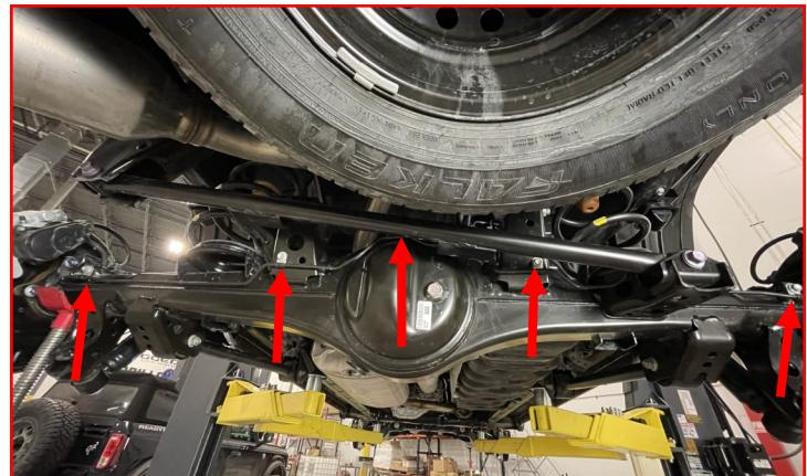
Remove the **bolt** (one on each side) holding the brake line to the axle.
