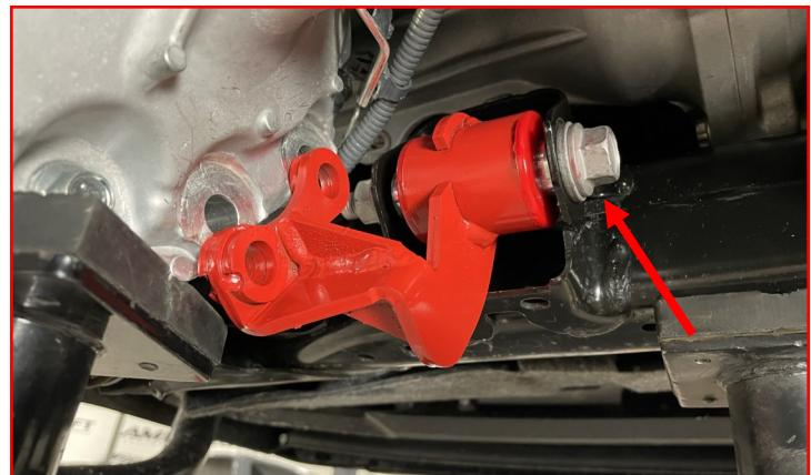
Install the supplied M14-1.5 x 60 SHCS and M14 flat washer into the upper differential mounting hole.
