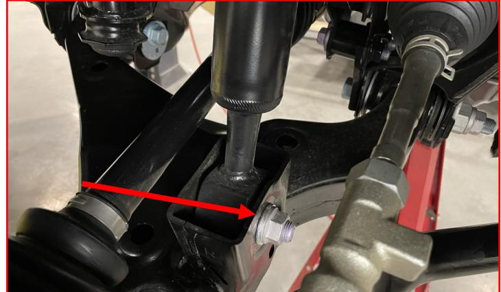
Remove the four (4) upper strut bolts.
