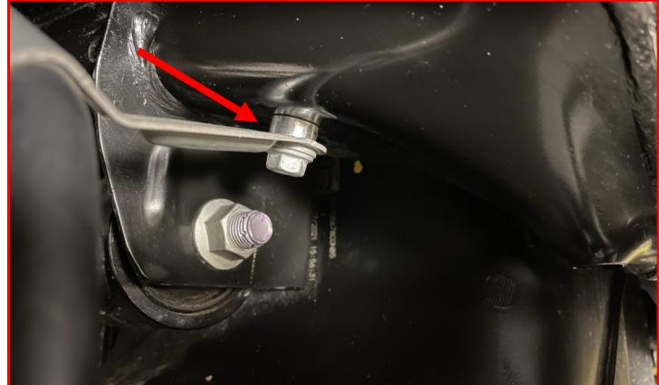
Using **factory hardware**, install the rear **brake line relocation bracket** holding the brake line to the frame.
