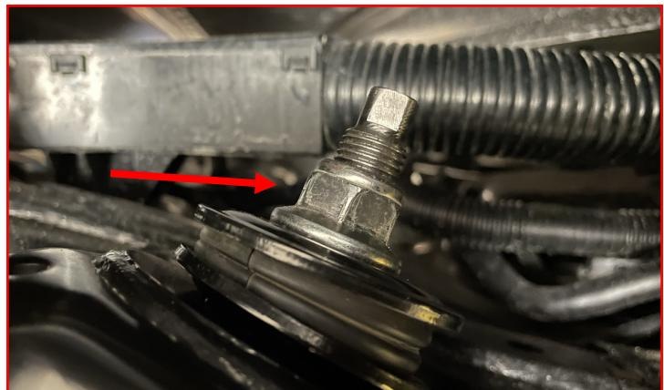
Torque the **lower shock bolt** to **60 ft-lbs**.
