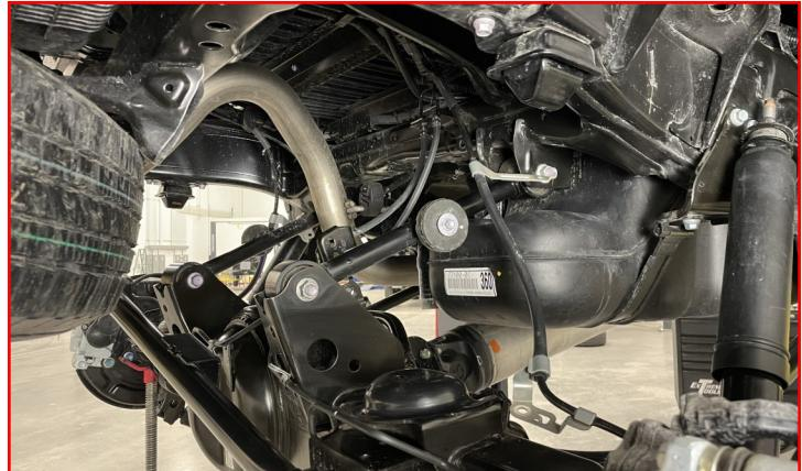
Place the ReadyLIFT **rear spring spacer** on the top of the factory bump stop and spring assembly as shown.
