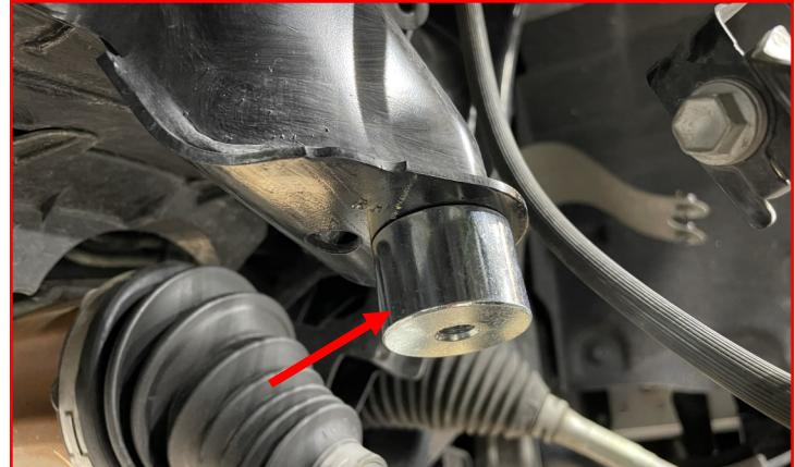
Attach the **factory bump stop** to the supplied extension.
