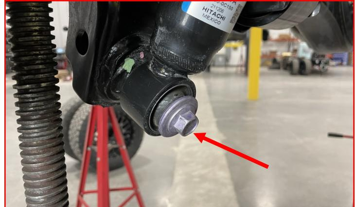
Remove the **upper shock nut** and **bushing**.
