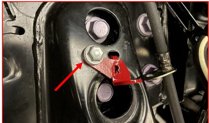
Attach the brake line to the **brake line bracket** using **factory hardware** and the supplied **M8-1.25 locking nut** and **M8 washer**.
