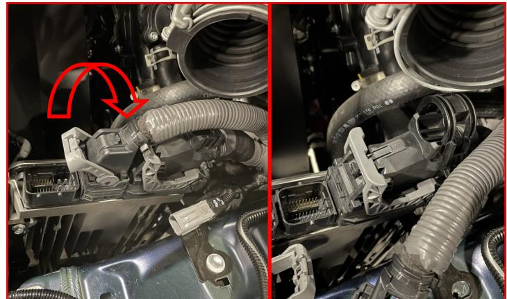
Clip the **factory hose clip** onto the wire housing for the center plug.
