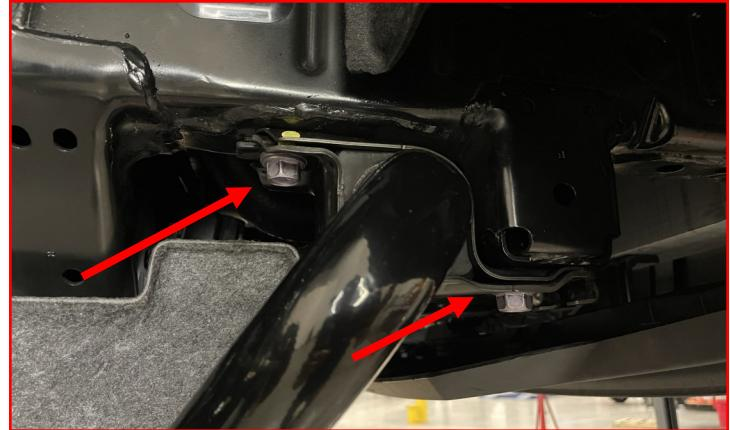
Remove the **sway bar end link bolt** from the lower control arm and slide the **end link** off of its perch.
