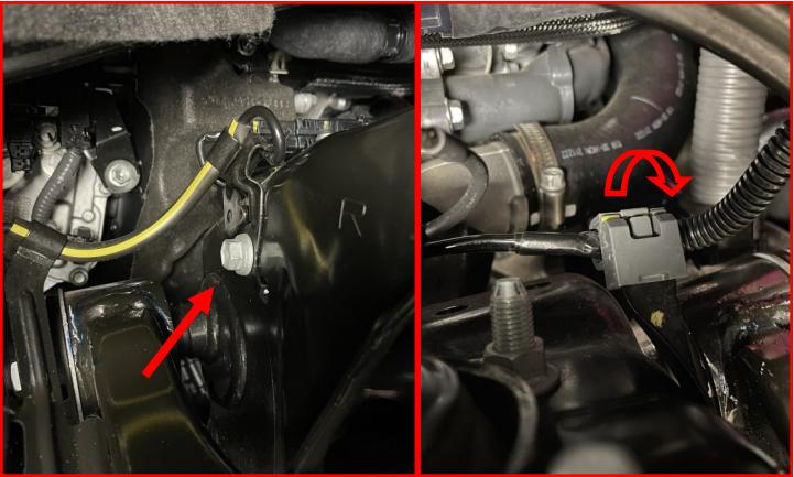
Release the AVS plug from the bracket by gently **pulling up** on the tab and **sliding** the bracket out of the plug.
