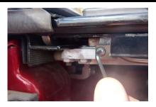
Locate the Allen head screw. It is a 3/32 screw holding the lock rod onto the lock assembly. This screw will need to be removed.
