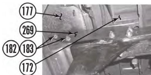
c. Adjust rear bumper (177) to bed (172) clearance using measurements from step B.13.a. Tighten nuts (179 and 182) to 55 lbs-ft.
