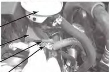
f. Remove wire harness (94) from clip (95) on passenger side wheel well (67) behind power steering reservoir (88).
