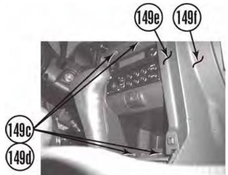
e. Position shift lever console (149a) on storage console (149b) and install manual shift knobs (146 and 147) on manual shift levers (148 and 149).
