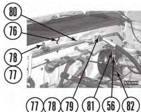
d. Check AC line (80) at the core support (14) for ample slack. If necessary carefully bend AC hard line downward to gain slack.
