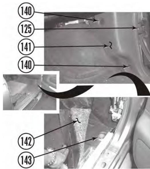
c. Pull carpet (142) back and expose two plastic bolt lockers (143).
