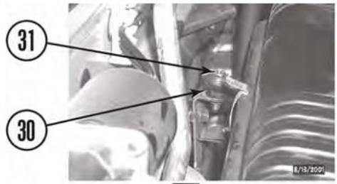
d. Remove two wing nuts (32) and five clamps (33) from air cleaner housing top (30) and throttle body (34).
