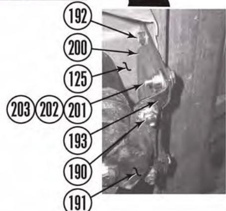
5. Finish cab spacer block installation.
