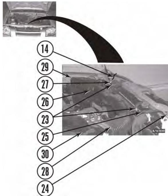
c. Remove bolt with captive washer (31) from air cleaner housing top (30).
