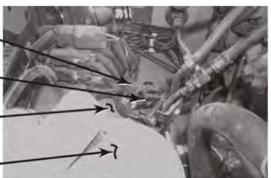
g. Remove clip (113) and ground strap (114) from passenger side wheel well (67).
