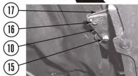
e. Remove two bolts (18) and front outer bumper (10) from two side front outer bumper braces (19).
