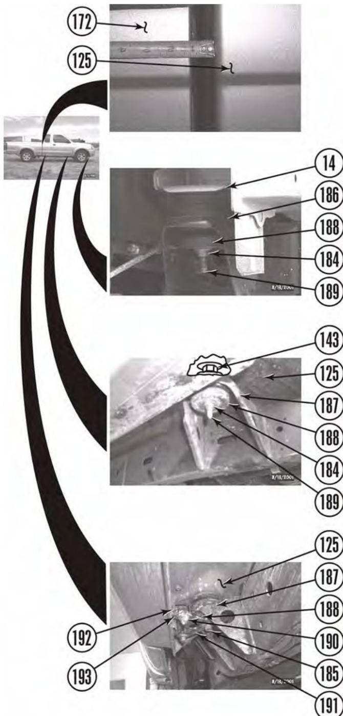
2. Lift cab and install passenger side spacer blocks.
