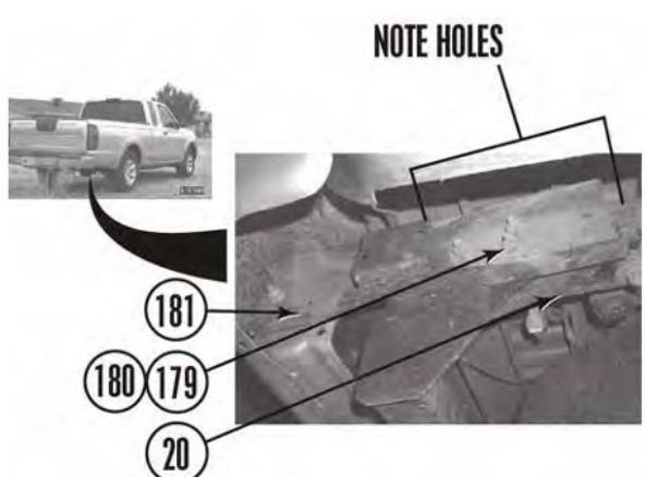
d. Remove rear bumper (177) and rear bumper brackets (181) from frame (20).
