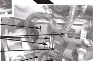
j. Remove two bolts (118) and bracket (116) from fire wall (76).
