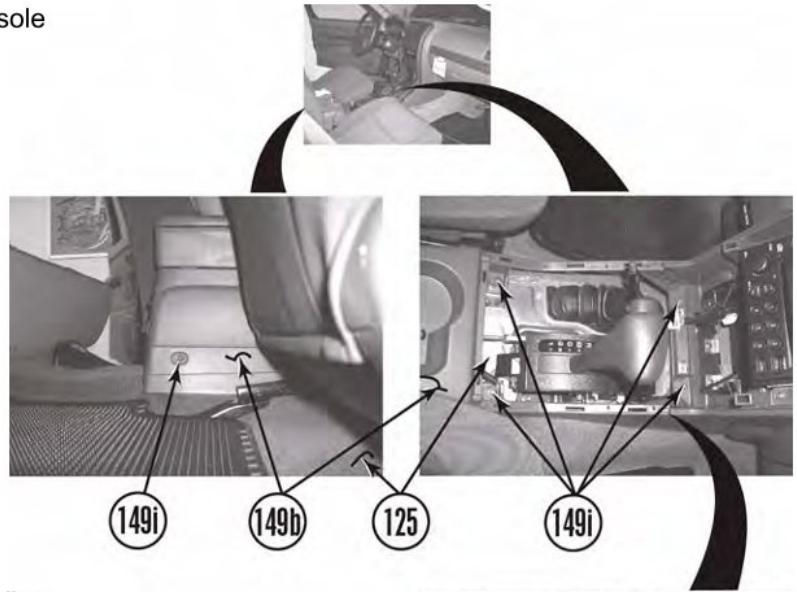
f. Lift storage console (149b) and locking clips (149j) from dash (149f).
