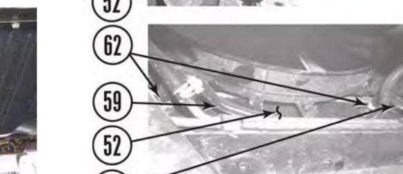
l. Remove two hose clamps (62) and transmission cooler hoses (59 and 63) from radiator (52). Plug transmission cooler hoses.
