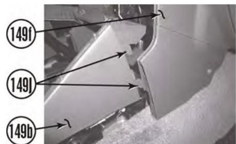
b. Install storage console (149b) on cab (125) with six screws (149i).
