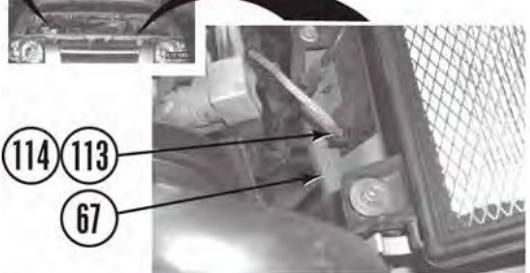
l. Remove two bolts and bracket from airbox and wheel well.
