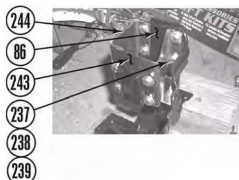
e. Install power steering bracket (86) on passenger side wheel well (67) with two bolts with captive washers (87) and two nuts (85).
