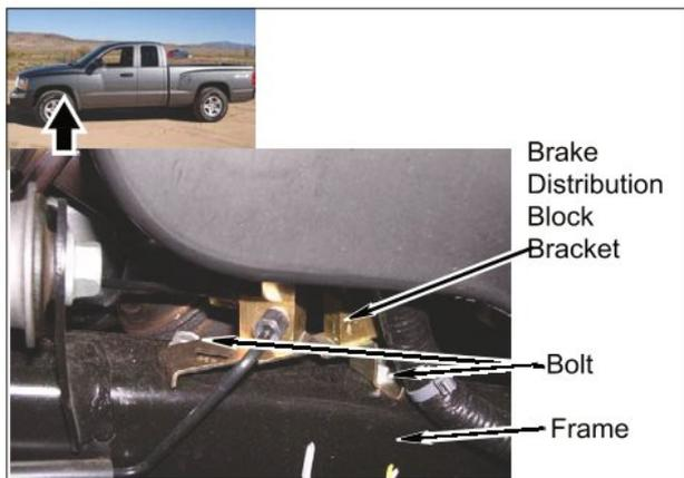
b. Remove bolt, ground wires, and clip from frame.
