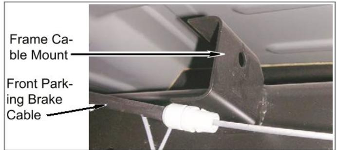
c. Remove brake line from clip on frame.
