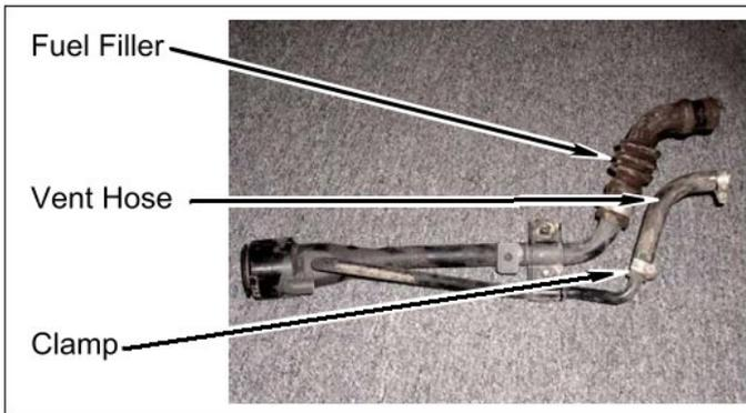
d. Install **kit hose** (1/2" x 11") onto fuel filler vent tube with **kit clamp** (#10 hose).
