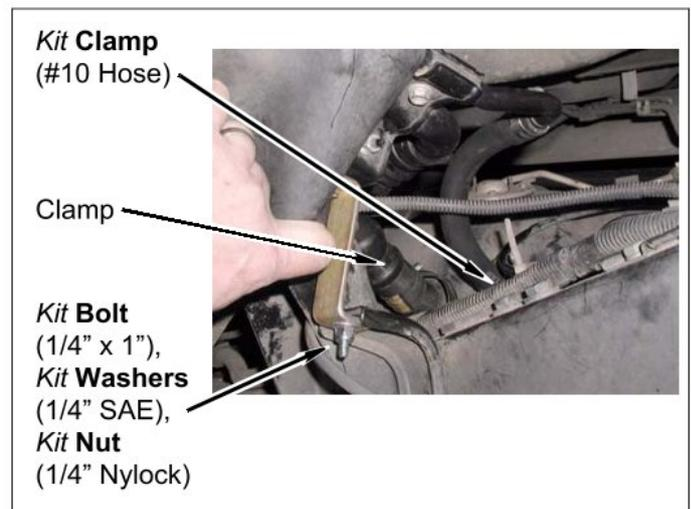
i. Install **kit bracket** (3" Z-shaped) onto frame bracket with **kit bolt** (1/4" x 1"), two **kit washers** (1/4" SAE), and **kit nut** (1/4" Nylock).
