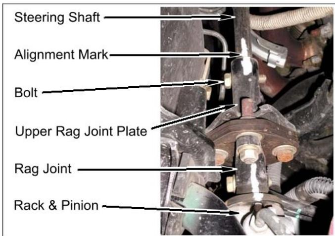
c. Remove bolt and slide steering shaft up off rag joint.
