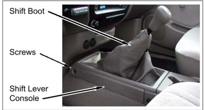
k. Install rear center console onto shift lever console with four bolts and two screws.
