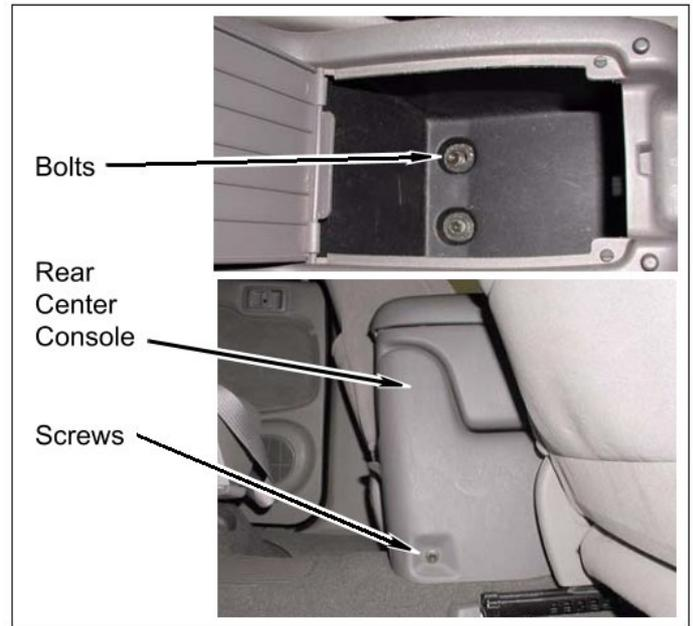
c. Remove two screws from shift lever console.
