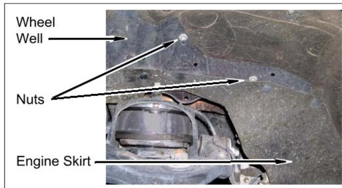
b. Remove push clips and three engine skirts from driver and passenger side front wheel wells.
