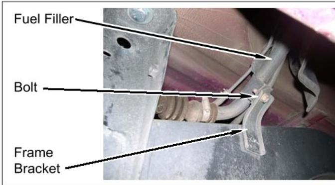
b. Loosen two hose clamps at fuel tank and remove fuel filler from vehicle.
