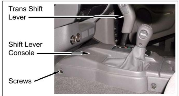
h. Install rear center console onto shift lever console with four bolts and two screws.
