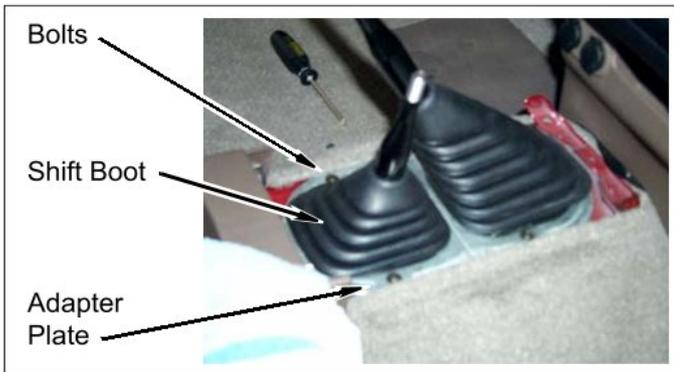
j. Install outer transmission shift lever boot and shift lever console with two screws.
