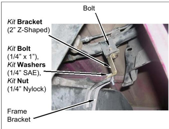
j. Install **kit bracket** (2" Z-shaped) onto frame bracket with **kit bolt** (1/4" x 1"), two **kit washers** (1/4" SAE), and **kit nut** (1/4" Nylock).
