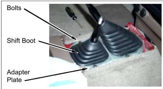
e. Lift lower transmission shift lever boot and press locking collar down around transmission shift lever. Turn locking collar counterclockwise and remove transmission shift lever, lower boot, locking collar, and spring from transmission.
