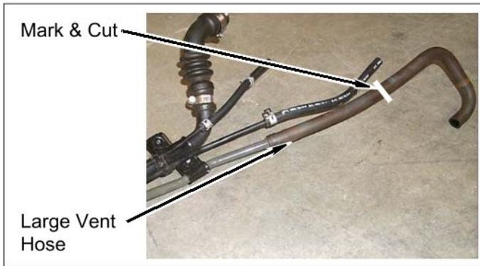
h. Install **kit extension** (5/8" x 3", metal) between two cut sections of large vent hose with two **kit clamps** (#10 hose).
