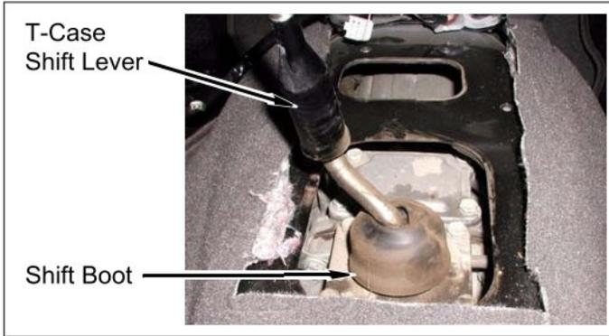
h. Install transmission shift lever, lower boot, locking collar, and spring onto transmission.
