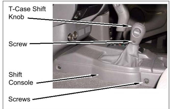
b. Remove four bolts, two screws, and rear center console from shift lever console and vehicle.
