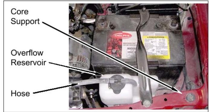
3. Remove two bolts and positive battery cable from driver side front wheel well and frame.
