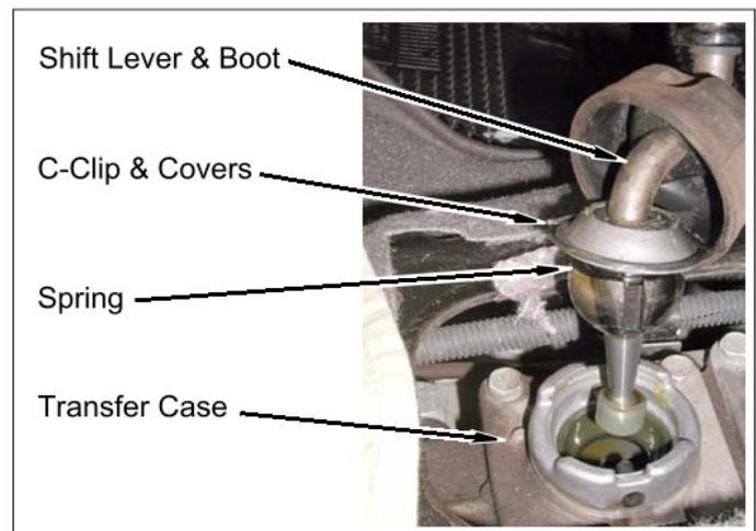
g. **Manual transfer case models:** Install lower transfer case shift lever boot onto transfer case.
