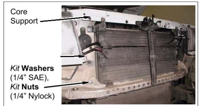
3. Install radiator overflow reservoir onto core support and connect overflow hose.
