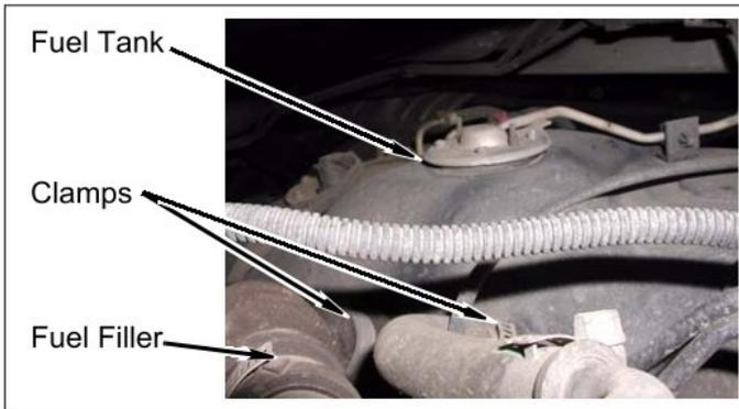
c. Remove clamp and vent hose from fuel filler assembly.
