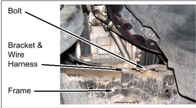
3. Remove clip and parking brake cable from driver side frame bracket.
