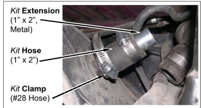
f. Install **kit extension** (1" x 2", metal) into **kit hose** (1" x 2") with **kit clamp** (#28 hose).
