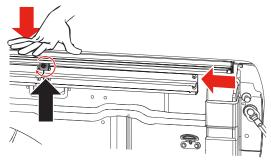
Place the third clamp (H) near the rear of the rail, approximately 12" from the tailgate. Hand tighten to 10 ft/lbs of torque with a 1/2" wrench or socket. For trucks with cargo rails, the rear clamp should be positioned as shown here, between the cargo rail and the truck bed flange. Repeat steps 2-5 on the driver's side rail (B).
