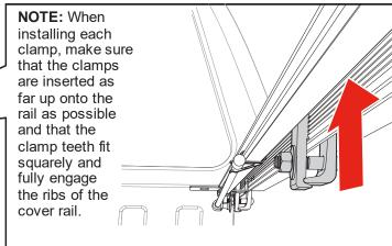
Place the second clamp (G) near the center of the rail. For 8' beds, two clamps will need to be evenly spaced in the center section of the rail. Hand tighten to 10 ft/lbs of torque with a 9/16" wrench or socket.
