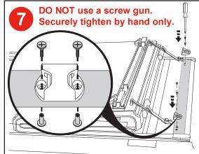
Position the buckle ends (N) so the open side faces the bed cover panel. Use a screwdriver to install the two buckles into the pre-drilled holes on the front head er panel with the provided machine screws (O) and rivet nuts (P).
