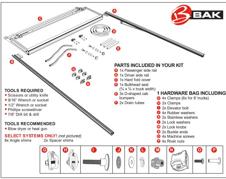
Clean the top of the bulkhead to install the seal (D). Peel the backing and adhere the seal from one bedrail edge to the other. Remove any excess with scissors or a utility knife. If the truck has a drop-in bedliner, no seal will be needed.
