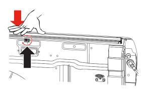
FOR TRUCKS WITH CARGO RAILS: Insert the second clamp (G) above the cargo rail near the tailgate. Slide the second clamp to near the center of the cover rail. For 8' beds, two clamps will need to be evenly spaced in the center section of the rail. Hand tighten to 10 ft/lbs of torque with a 9/16" wrench or socket.
