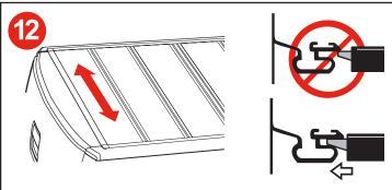
Check to see that the cover panel latches make proper contact with the side rails. If adjustments are needed, loosen the lock knobs (M) and shift the cover slightly until proper latch engagement is achieved. Then retighten the lock knobs.
