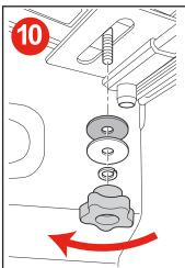
Assemble the washers from underneath and **loosely** tighten the knob (M).
