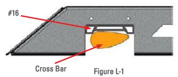
Repeat this process to add rubber clamp (#16) on the opposite side. Check that there is no contact with the roof, the moon roof (in any open or closed positions), any roof mounted antenna, or the lift gate/hatch (in any open or closed positions). If any contact occurs, adjust the height of the rack from the roof, the expanded length of the rack, or both. *If no adjustments are needed skip to Step 15. Otherwise, continue to next step.*
