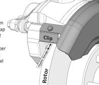
Caliper Cover should rest directly against the face of the brake caliper. The installer should verify that the bridges are set to 88°as depicted on image. Installer may adjust as needed.
