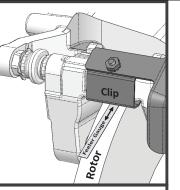
Caliper Cover should rest directly against the face of the brake caliper. The installer should verify that the bridges are set to 88°as depicted on image. Installer may adjust as needed.
