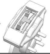
Caliper Cover should rest directly against the face of the brake caliper. The installer should verify that the bridges are set to 88°as depicted on image. Installer may adjust as needed.
