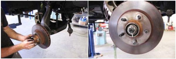
Slide the brake caliper back onto the spindle, place several drops of thread lock / locktite onto the original brake caliper bolts and attach the caliper to the spindle. Torque bolts t 35 ft/lbs.
