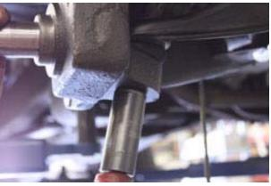
Slide the rotor back onto the spindle, install the original castle nut and adjust preload on wheel bearing to factory spec. It's important to check the clearance between the ABS Sensor and the relluctor ring. If there is contact, refer to previous step to space the sensor back.
