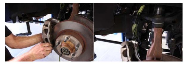
Support the lower control arm with a floor jack, compress the arm ¼". Remove the cotter pin and castle nut from the tie rod end at the spindle. Separate tie rod end from the spindle, then remove the dust cap from the rotor. Slide the rotor and bearings off the spindle.
