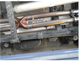
**Step 4:** Loosely install the Mid Pipe Assemblies by attaching the inlet ends to the outlets of the X-Pipe Assembly. The Pipe assembly with the welded hanger goes on the passengers side. Locate the welded hanger to the rubber insulator.
