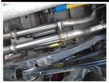
Step 5: MagnaFlow supplies this kit with multiple build options giving the ability to use different muffler, NDT and muffler deletes depending on preference.
