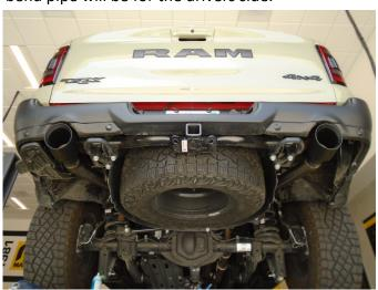
**Step 8:** Loosely attach each Tail Pipe Assembly to the Tailpipe Extension Pipes using the supplied clamps. Locate the welded hangers to the rubber isolators.
