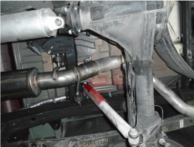
Step 5. Slip the Outlet Resonator exit pipe over the cut OEM rear pipe. Loosely secure using the supplied band clamp. Engage the welded hangers to the rubber insulators.
