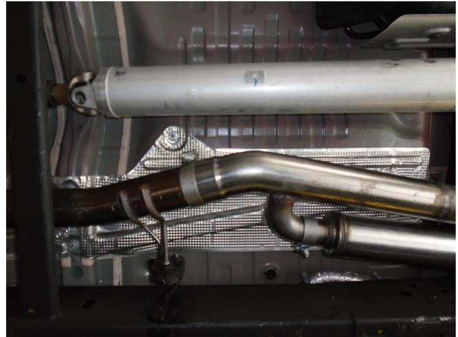
Step 3. Begin installation by slipping the inlet of the Inlet Resonator Assembly over the cut OEM outlet pipe. Secure using the supplied band clamp. Keep all clamps loose until the final assembly is complete to allow for adjustment.
