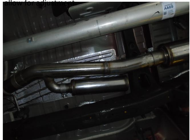
Step 4. Install the Outlet Resonator Assembly by attaching the inlet pipe to the outlet of the Inlet Resonator Assembly. Loosely secure using the supplied band clamp.
