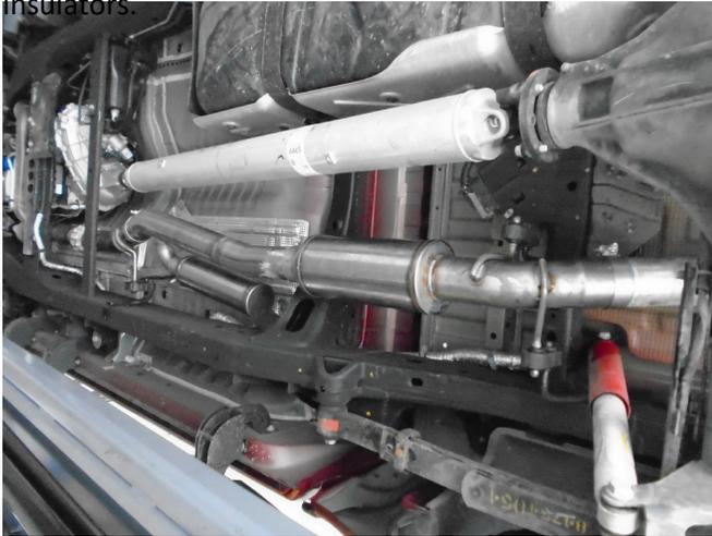
Step 6. With the new MAGNAFLOW system in place all loose band clamps can now be tightened. Your installation is complete.
