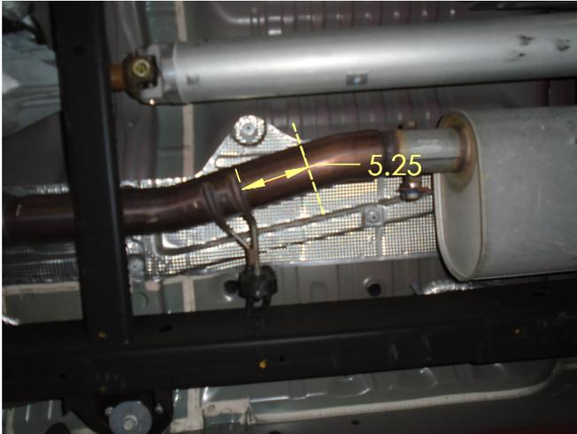
Step 1. The muffler section will need to be removed from the OEM exhaust system. Using a Sawzall or similar cutting tool cut the exhaust pipe 5.25" rearward of the welded hanger in front of the muffler.
