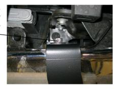
13. PLACE THE TOP MOUNTING BRACKET (ITEM #4 OR #5) IN POSITION AND REINSTALL THE BOLT AND SNUG UP. IF THE GUARD HAS THE OBROUND HOLES IN IT FOR THE TOP BRACKETS, FASTEN THE ENDS OF THE BRACKETS TO THE UPRIGHT WITH THE 1/2"-13 X 1-1/4" CARRAGE BOLT (ITEM #9), 1/2"-13 ACORN NUT (ITEM #11), TWO 1/2" FLAT WASHERS (ITEM #13) AND 1/2" SAE LOCK WASHER (ITEM #14). TIGHTEN ALL OF THE FASTENERS. REPEAT THE ABOVE ON THE OTHER SIDE.
