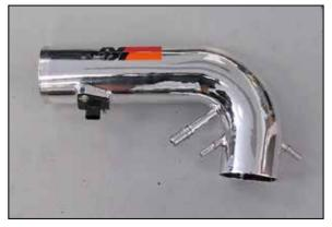
19. Install the mass air sensor into the K&N<sup>®</sup> intake tube and secure with the provided hardware.
