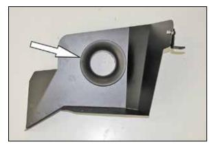
12. Install the provided filter adapter into the heat shield as shown and secure with the provided hardware.
