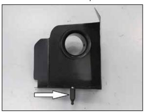
8. Install the heat shield mounting stud onto the bottom of the heat shield as shown.
