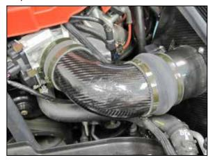
18. Install the K&N® intake tube assembly into the silicone hose at the throttle body and then install the hump hose onto the mass air sensor housing. Secure the tube with the provided hose clamps.
