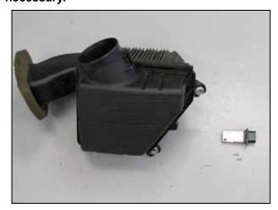
11. Remove the two screws securing the mass air sensor into the factory air box and then remove the sensor from the air box.
