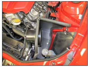
13. Install the heat shield into the engine compartment so the mounting stud inserts into the air box mount grommet and the mounting bracket installs onto the mounting stud.
