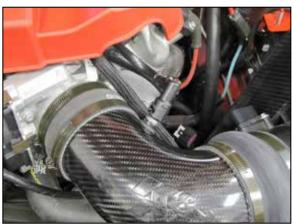
20. Rotate the crank case vent fitting clockwise and then connect to the fitting installed into the K&N® intake tube in the previous step.
