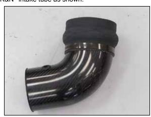
16. Install the provided hump hose (08695) onto the K&N® intake tube and secure with the provided hose clamp.
