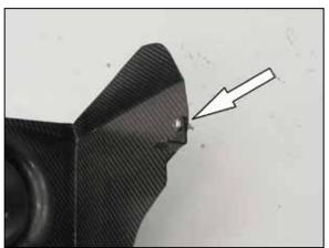
9. Install the heat shield mounting bracket (070066) onto the heat shield as shown.
