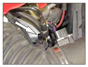
3. Disconnect the crank case vent from the intake tube.
