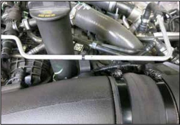
19. Secure the coolant by-pass line to the bracket with the provided mounting cable tie.
