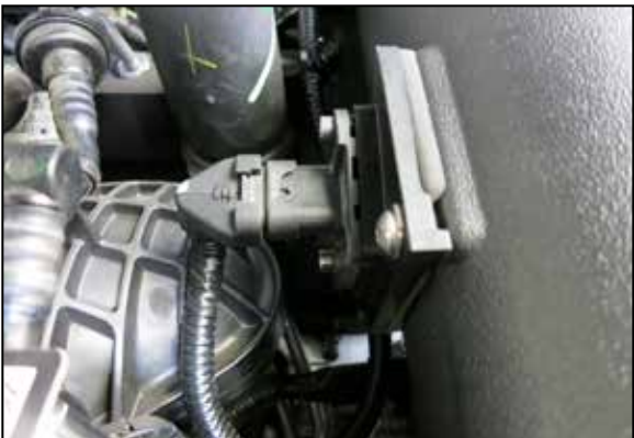
18. Reconnect the mass air sensor electrical connection.
