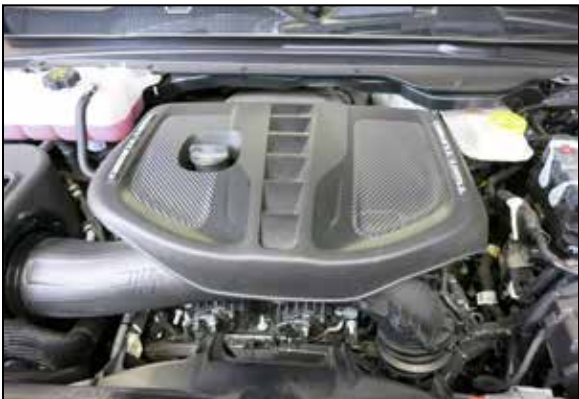
20. Reinstall the engine cover and secure with the factory mounting bolt.
