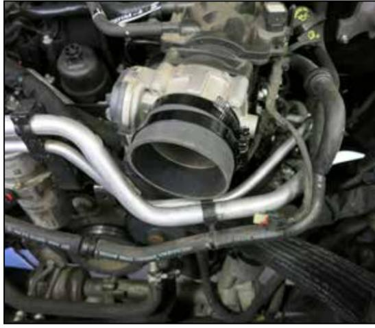
8. Install the provided coupler onto the throttle body with the hose clamps. Tighten clamps using 5/16" socket or nut driver.
