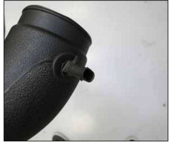
13. Remove the IAT sensor from the factory intake plenum, remove the O-ring from the sensor and then install it into the K&N intake tube with the provided grommet.
