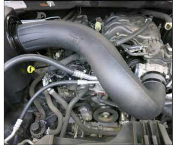
14. Install the intake tube into the air filter and then into the coupler on the throttle body, adjust the tube for best fit and secure with the hose clamps. Tighten clamps using 5/16" socket or nut driver.
