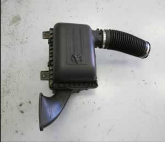
5. Lift the air filter housing up to dislodge it from the mounting posts and then remove it from the vehicle.
