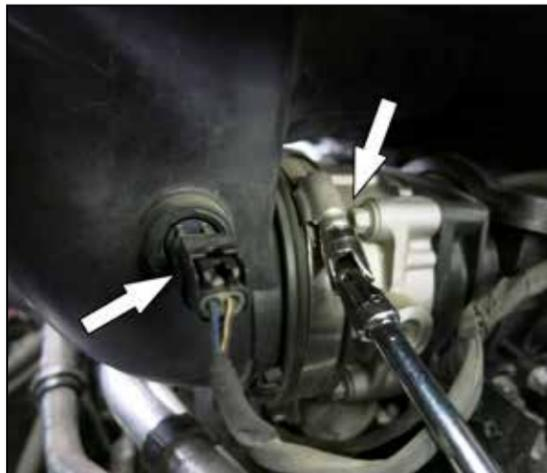
2. Disconnect the IAT sensor electrical connection and loosen the hose clamp that secures the intake plenum to the throttle body.
