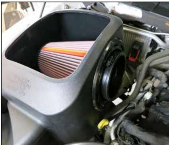
12. Install the K&N air filter into the K&N air filter housing.
