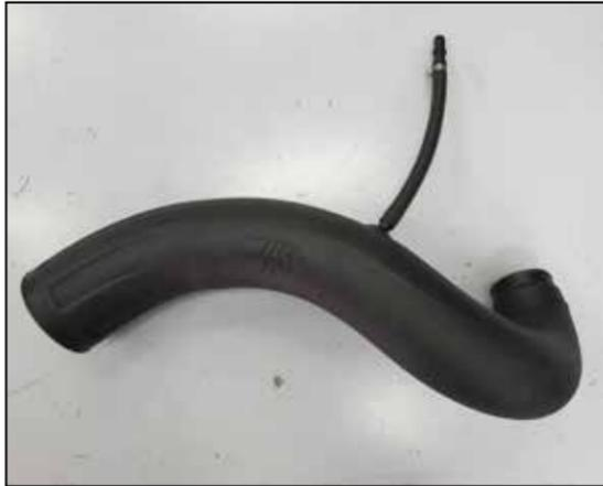
10. Install the CCV hose assembly into the K&N intake tube as shown.
