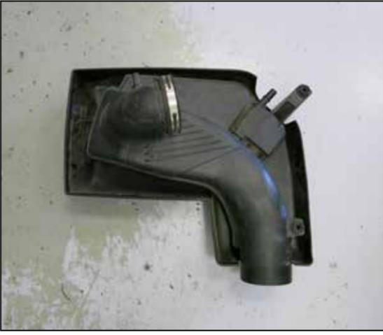
4. Unhook the intake plenum from the mounting posts, then the throttle body and remove it from the engine.
