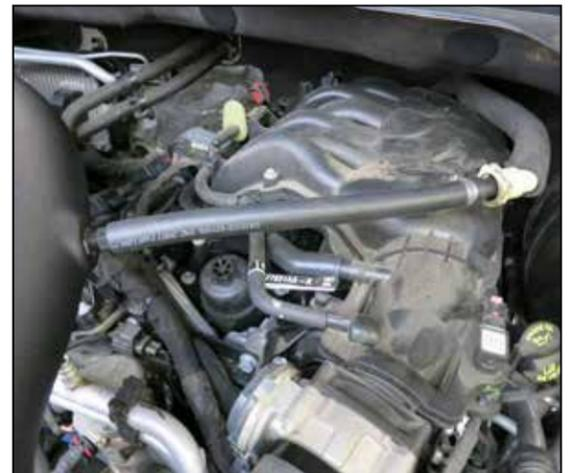
15. Connect the CCV hose quick connect fitting into the factory CCV fitting.
