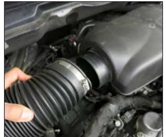
3. Loosen the hose clamp that secures the intake hose to the intake plenum and then disconnect the hose.
