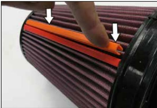
11. Attach the filter clips to the pleats on the air filter align and push down. Passenger side filters, place orange clip on top and red on bottom.
