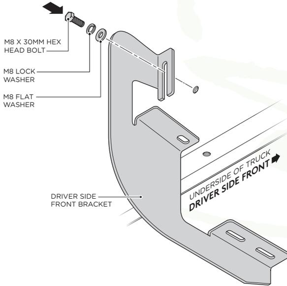
5. Fasten the bottom portion of the Driver Side Front Bracket by using (1) M8 x 30MM Hex Head Bolt, (1) M8 Flat Washer and (1) M8 Lock Washer.
