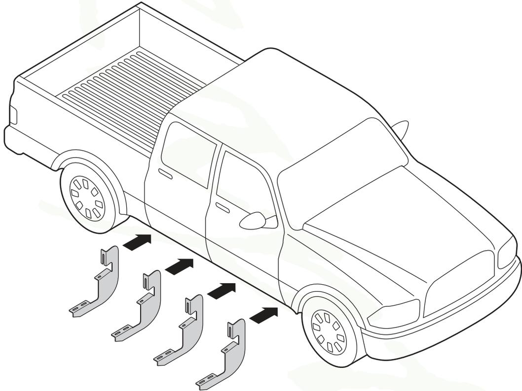
2. Passenger Side Front Bracket cradle (2a), Passenger Side Center Bracket cradles (2b, 2c), and Passenger Side Rear Bracket cradle (2d) will all face towards the rear of the truck.
