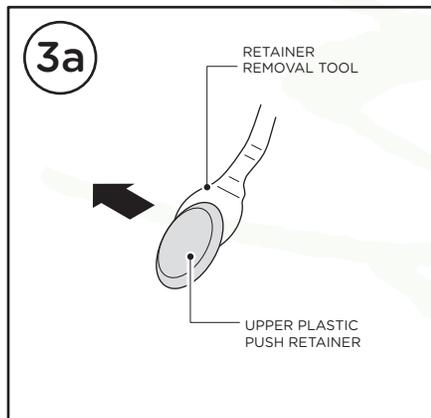
Pull the upper Plastic Push Retainer out of the rocker panel to expose threaded holes that will be used for bracket installation.
