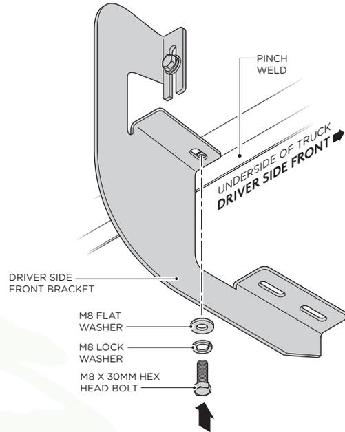
6. Fasten the top portion of the first Driver Side Center Bracket by using (1) M8 x 30MM Hex Head Bolt, (1) M8 Flat Washer and (1) M8 Lock Washer.
