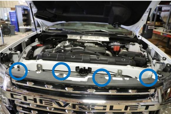
9. Remove grille and detach front camera cable (if equipped). You will remove the camera at this time and connect the [camera cable extender \(sold separately\)](#).
