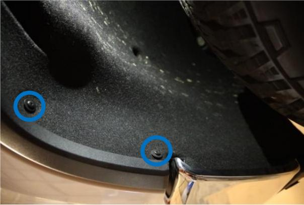
2. Remove fender flare and remove one 7mm bolt
