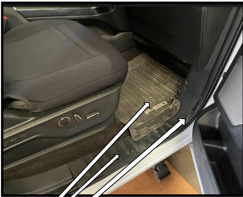
Remove drain plug, A-pillar, Sill Panel, b-pillar trim and carpet
