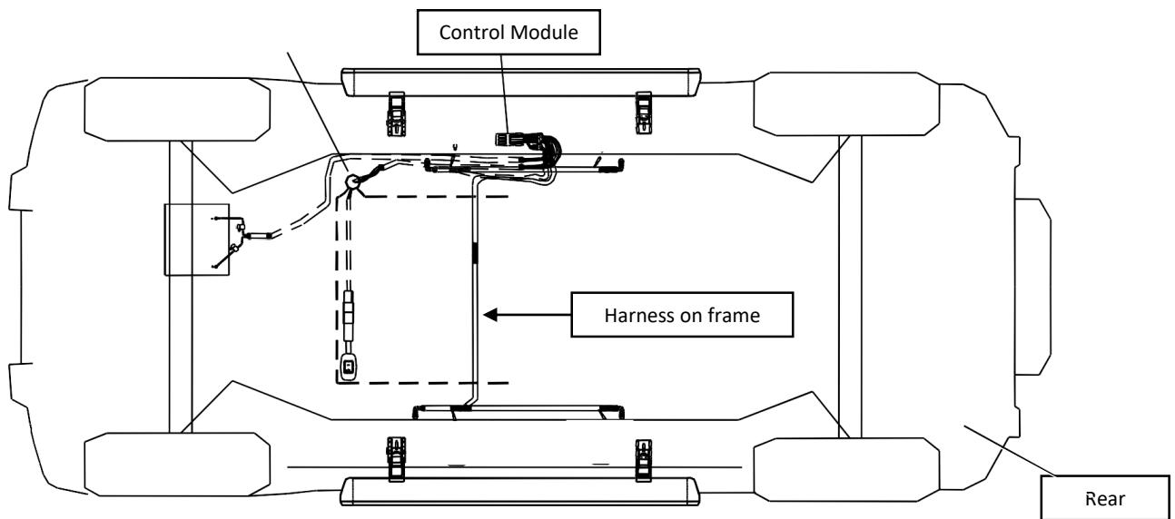
**Step 12:** Route the motor wire harness from the controller to the Passenger side frame rail of the vehicle. When routing the harness keep clear from any moving parts and avoid direct contact with the exhaust system.
