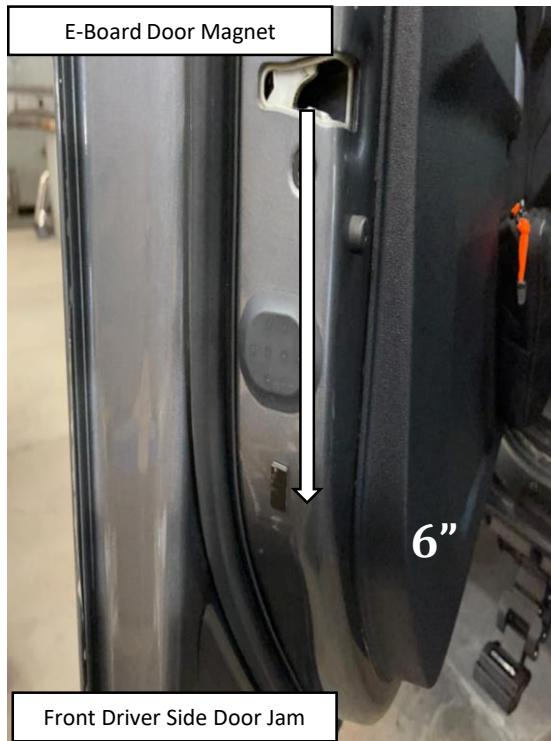
**Step 16: FRONT DOOR** Apply a vertically oriented strip of masking tape on the front driver side door using the deepest part of the latch as a reference point. Make a mark 6" below the center line of the latch. Prepare the surface by cleaning with a 50/50 mix of isopropyl alcohol and water or equivalent. Once the surface is completely dry, peel the backing from the double-sided tape and stick the magnet to the door. Align the top of the magnet with the 5" mark as shown.
