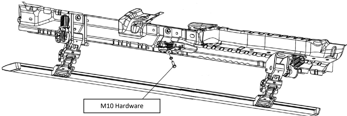
**Step 5:** Locate the threaded holes near the center of the cab on the Driver side of the vehicle. Install the controller bracket using (2) M10x25MM hex bolts M10 Lock Washer, M10 Flat Washer, to fasten the control module to the vehicle.
