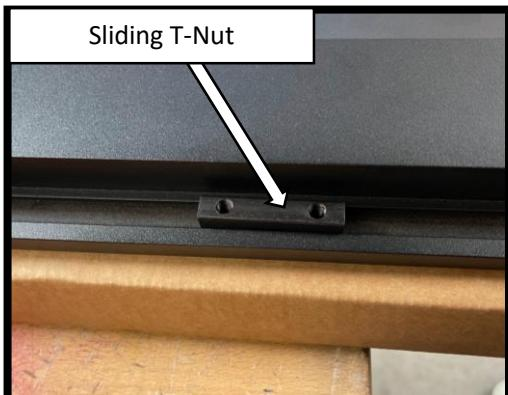
**Step 6:** Install the driver side running board. With assistance, begin by positioning the board on the front and rear motor assembly bases. Align the sliding T-Nut on the running board with the slots on the front and rear motor base. Once the T-Nuts are aligned, rotate the running board so that the T-Nuts set in the slots on the base of the arms. Repeat Steps 3-6 to install the motor linkage assemblies and running board on the Driver side.
