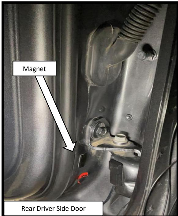
**Step 20:** Repeat steps 14-19 to install the Passenger side door trigger sensors and magnets. The Passenger side door trigger harness is connected to the white wire that was routed under the carpet to the Passenger side b-pillar in Step 13
