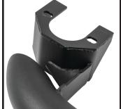
On the body mount remove the 2 nuts on either side of the mount.
