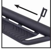
Carefully place HS2 step onto Place. Secure mounting holes over OE studs. Best to have a assistant to lift and hold board in place. Now hand tighten nuts to OE studs.
