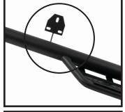
Remove OE boards if equipped then locate mounting holes. Insert U nuts to the bottom two holes
