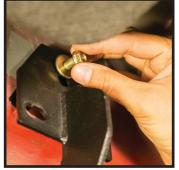
Begin tightening nuts & bolts in a alternating pattern. Avoid using power or air tools. Tighten to 20ft lbs torque to secure the board to the truck. Repeat the same procedure to the other side.
