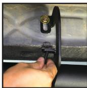
**STEP 4** (Drivers Side): Carefully place HS2 step into place. Use bolt, washer and begin hand tightening all 4 upper mountings. Best to have a assistant to lift and hold board in place.
