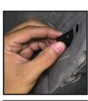
**STEP 3:** Insert spring loaded U nuts to the body of the truck.
