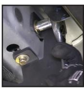
**STEP 6: Avoid using power or air tools.** Tighten lower mounting first then upper bolts. Tighten to 20ft Ibs torque to secure the board to the truck. Repeat the same procedure to the other side.
