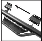
Carefully place HS2 step onto the studs. Add washers and begin hand tightening nuts. Best to have a assistant to lift and hold board in place.
