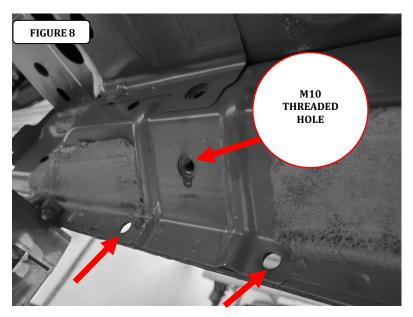
**Step-6** Attach the driver side Rear bracket to the pinch mold using (2) 1/4" x 1" hex head bolts, (4) 1/4" flat washers, (2) 1/4" lock washers and (2) 1/4" hex nuts, and to the underside of the body using (1) M10 x 25mm hex bolt, (1) M10 lock washer and (1) M10 flat washer, (FIGURE 9 & 10). Leave the nuts and bolts loose for final adjustment.
