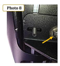
**Step-9** Align the side step with the vehicle and tighten all brackets and side steps nuts and bolts. Repeat the above steps to install the passenger side brackets and side step. Remember to check and retighten the nuts and bolts every six months.
