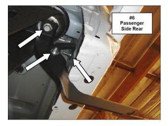
Step-7 Insert the bolt shim assembly into the rails of the inner aluminum extrusion at the underside of the side step. Each side step requires (6) M8 x 25mm. Hex bolt, 2 at the front, 2 at the rear, and 2 at the middle
