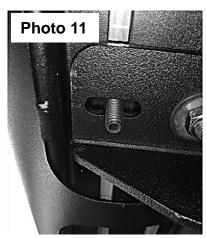
Step-9 Align the side step with the vehicle and tighten all brackets and side steps nuts and bolts. Repeat the above steps to install the passenger side brackets and side step. Remember to check and retighten the nuts and bolts every six months.
