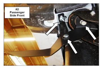
**Step-3** Remove the passenger side middle body mount bolt. Keep all existing bushing in place, and attach the passenger side middle bracket to the vehicle using the factory body mount bolt, (Photo 3 & 4). Leave the body mount bolt loose for final adjustment.
