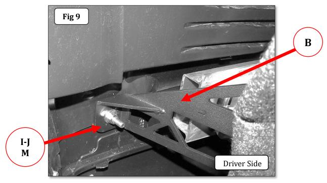
**Step-13** Use the (2) holes in the Lower Wrap HD side bracket as a guide and drill 7/16" holes through the wheel arch molding and bumper cover, (Fig 10).
