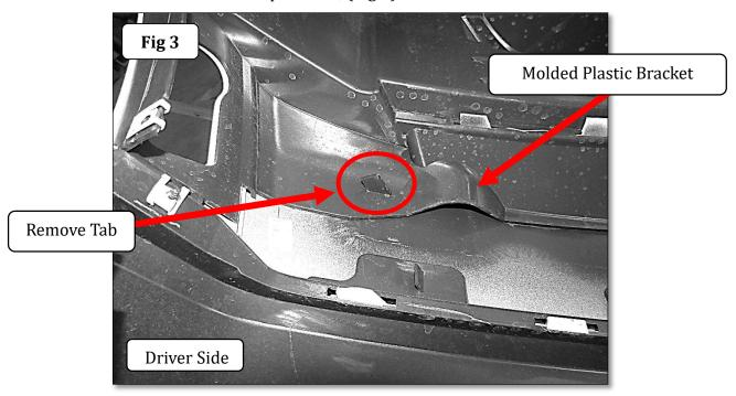
**Step-4** Reinstall the bumper cover. Note: Do not reinstall the fender inner liner and wheel arch molding at this time.
