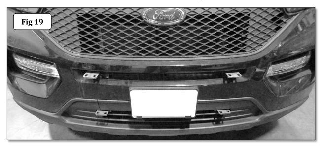
**Step-13** Attach the upper and lower extension brackets to the main brackets using (2) 3/8" X 1 1/4" hex bolts, (4) 3/8" flat washers, (2) 3/8" lock washers and (2) 3/8" hex nuts for each extension bracket, (Fig 20). Leave the nuts and bolts loose for final adjustment,
