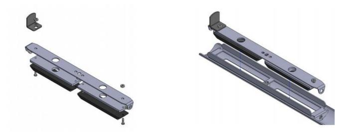
2. Place the light on top of the mask bracket and align it. Secure the assembly using (3) 1/4" x 3/4" allen head bolt See image 2 & 3.
