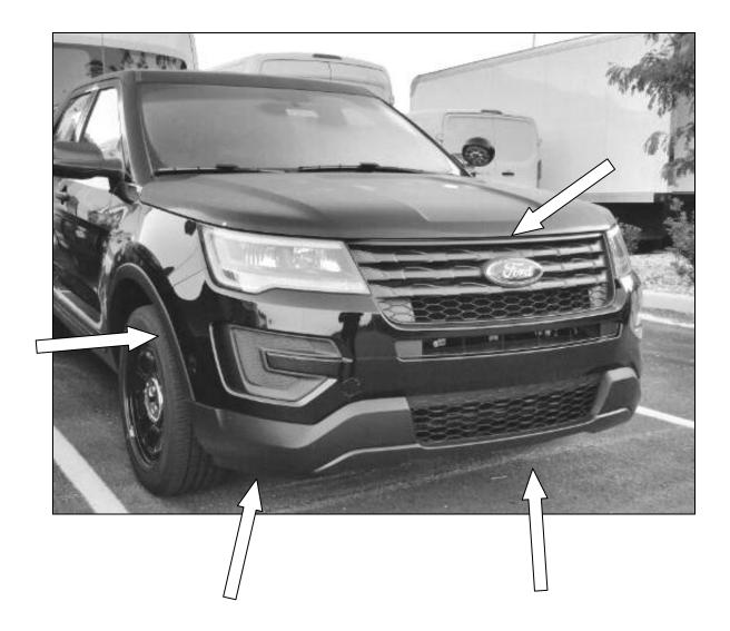
**Step-5** With assistance pull out on the sides to release the corners of the front bumper fascia and forward to remove it from the vehicle. **Note:** Unplug the fog lights if equipped.
