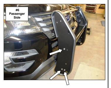
**Step-7** Use the front fender and bumper fascia seam as a reference point and measure downward from the upper edge along the seam 1 5/8" and mark a line on the bumper fascia. Use the marked line as a reference point and measure downward from the seam on a 90 degree angle and mark a line 3 5/8" long on the bumper fascia, (Photo 7). Repeat this step for the driver side.
