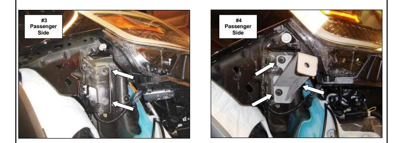
**Step-4** Reposition the front bumper fascia on the vehicle and install the hex bolts and plastic connectors securing the top of the fascia, install the hex bolts securing the fascia to the front fenders and the hex bolts securing the bottom of the fascia. Tighten all bolts. **Note:** Do not install the screws securing the fender liner and fender molding to the front bumper fascia.
