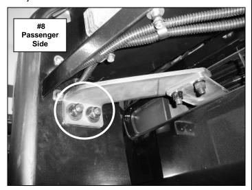
Step-9 Align the push bumper with the vehicle and tighten all nuts and bolts, (Photo 9 & 10).
