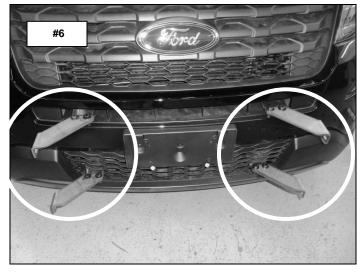
**Step-8** Attach the push bumper to each of the extension brackets using (2) 3/8" x 1" hex bolts, (2) 3/8" lock washers and (2) 3/8" hex nuts, (Photo 7 & 8). Leave the nuts and bolts loose for final adjustment.
