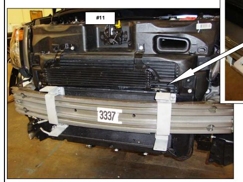
**Step-4** An area must be cut out from the back, of the top edge in the bumper fascia and bottom edge of the grille to allow clearance for the clamp brackets. Measure, cut and remove the outlined area from the bumper fascia and grille as shown, **(Photo 12 & 13).**
