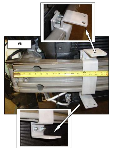
**Step-2** Assemble and attach the driver side main and clamp bracket to the steel impact beam using (4) 3/8" X 1 1/4" hex bolts, (4) 3/8" lock washer and (4) 3/8" hex nuts. Position the clamp bracket flush against the top of the impact beam and the outer edge approximately 11 3/4" from the end of the impact beam and tighten the nuts and bolts, **(Photo 9 & 10)**.
