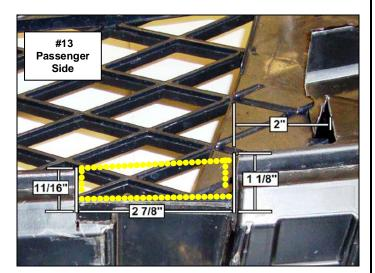
**Step-5** A section of webbing in each side of the lower grille must be cut out for the lower leg of the main brackets to extend through. Cut and remove the webbing from the lower grille as shown, **(Photo 13).**
