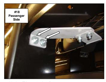
Step-9 Align the push bumper with the vehicle and tighten all nuts and bolts, (Photo 19 & 20).
