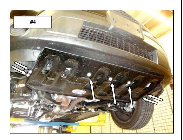
**Step-4** Remove the (9) hex bolts attaching the fascia to the core support and fender liner, **(Photo 5)**. **Note:** Photo shows the three passenger side bolts and two center bolts only.
