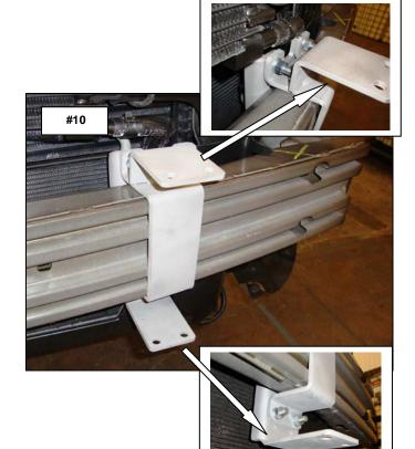
**Step-3** Reinstall the oil cooler bolts, check the bracket positions, and that the driver side bracket assembly does not interfere with the oil cooler lines.
