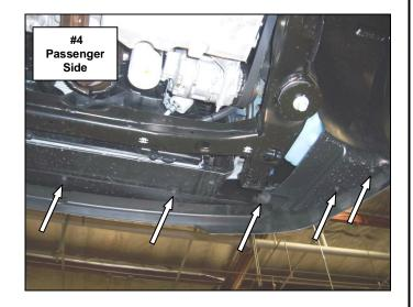
**Step-4** With assistance pull out on the sides to release the corners of the bumper fascia and forward to remove it from the vehicle. **Note:** Unplug the fog lights and parking sensors, if the vehicle is so equipped.
