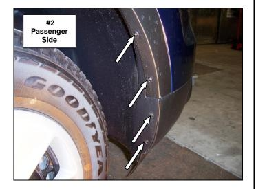
**Step-3** Remove the (9) hex bolts attaching the fascia to the core support and fender liner. Note: **Picture #4** shows the three Passenger side bolts and two center bolts only.
