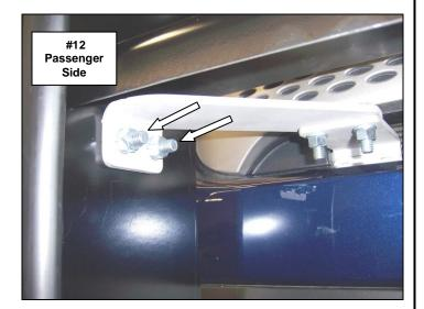
Step-6 Align the push bumper with the vehicle and tighten all nuts and bolts. Picture #13 & #14
