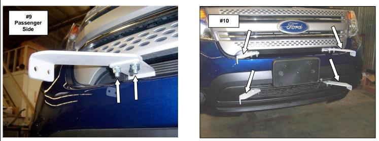
**Step-5** Attach the push bumper to each of the extension brackets using (2) 3/8" x 1" hex bolts, (2) 3/8" lock washers and (2) 3/8" hex nuts. Leave the nuts and bolts loose for final adjustment. **Picture #11 & #12**
